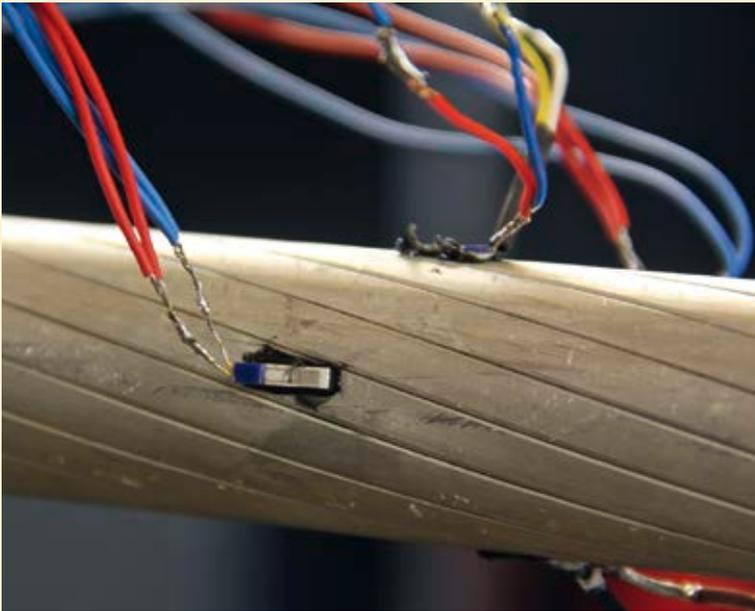
Fig. 4 The temperature sensors are fixed to the conductor with thermally conductive, high-temperature silicone adhesive.
