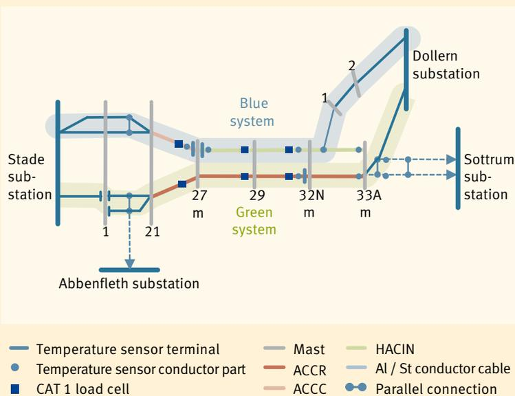
Fig. 5 Schematic showing the various types of conductors deployed during the field trial: HTLS conductors were used between masts 21 and 33A. The locations for the temperature measurements on the conductors are marked with a circle. The locations for the terminal temperatures are marked with a dash.
