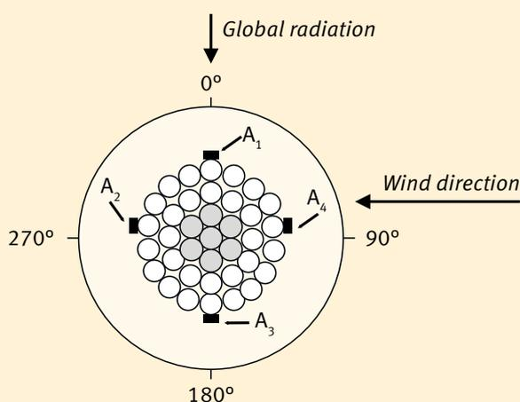
**Fig. 3** Precisely determining the conductor surface temperature was an important step in verifying the calculation models and identifying their inaccuracies. To achieve this, the researchers installed groups of four measuring sensors at specific intervals on the conductor with an angular displacement of 90°.
