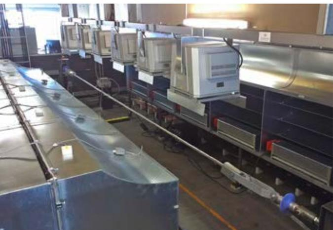
**Fig. 1** The laboratory rig enabled the researchers to simulate various weather conditions. The daylight bulbs above simulated the solar radiation, while the wind tunnel blew air at the conductor at an angle of 90°.
