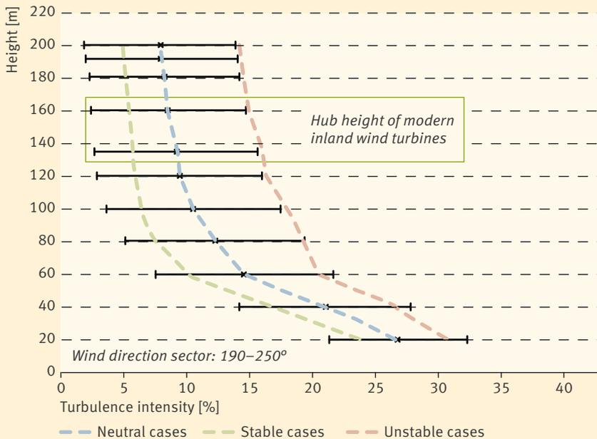
**Fig. 3** Dependence of the turbulence intensity relative to the height for the main wind direction sector on the 200-metre met mast. The turbulence increases considerably above the treetops. At the hub height of modern wind turbines, the turbulence intensity is comparable to offshore conditions with about 10%. Depending on the state of the atmosphere (stable, neutral, unstable), the turbulence increases considerably or attenuates.
