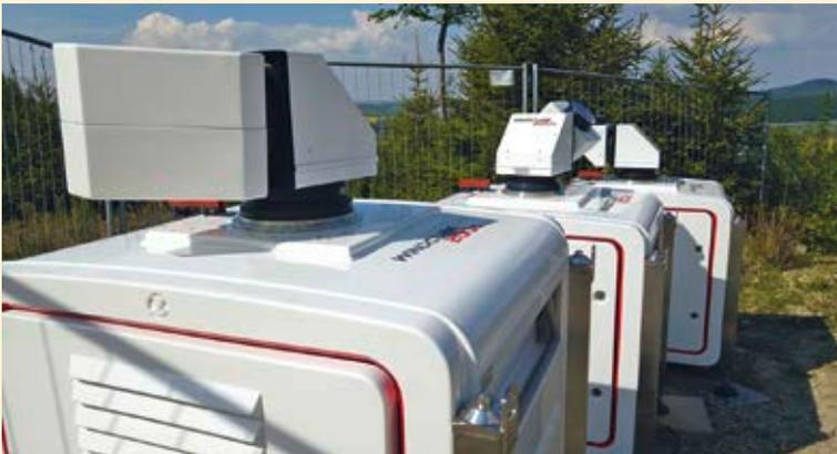
**Fig. 4** The measurements from these LiDAR devices were compared with the backup data from the met mast. This made it possible to identify systematic measurement errors and develop correction methods.
