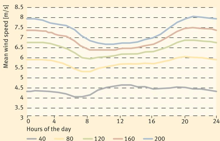
Fig. 2 During the day, the wind conditions above 120 metres and below 80 metres differ significantly.
