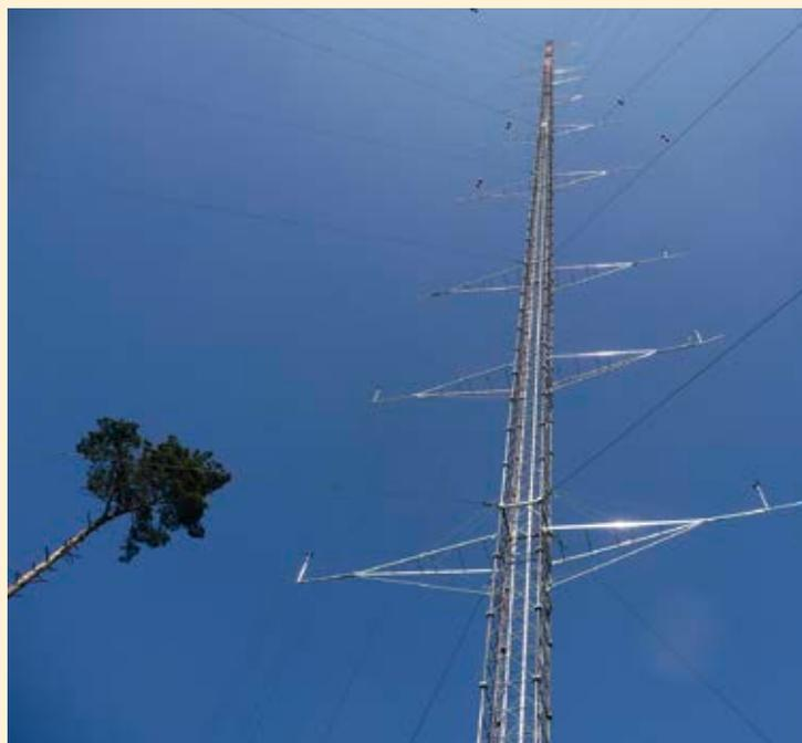
Fig. 1 The Rödeser Berg met mast is 200 metres high and is equipped with more than 40 instruments.
