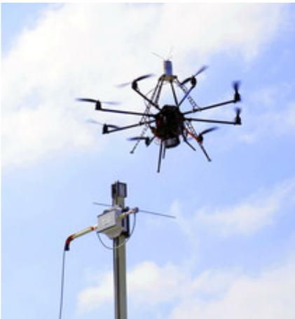
Using a so-called octocopter (pictured), the miniaturised system for measuring radar installations can fly through wind farms and carry out measurements at any point within the space.
