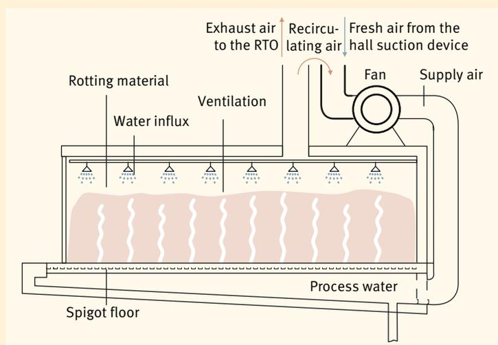
Fig. 2 Cross-section of the rotting box at the MBT Großefehn
