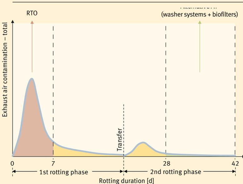
**Fig. 4** Carbon concentrations in the exhaust air during the course of the rotting process: initially exhaust air treatment using RTO, in the intermediate phase, depending on contamination, RTO and/or washers and biofilters; these are sufficient in the end phase.
