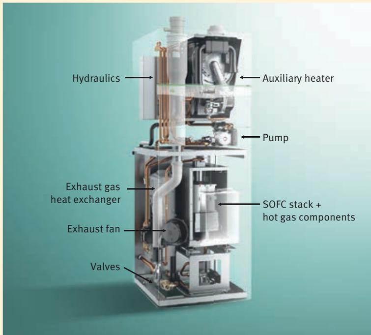
Fig. 4 Structure of the current XellPower FC heating appliance: the fuel cell system with the auxiliary units is below, the auxiliary condensing gas boiler heater is above.
