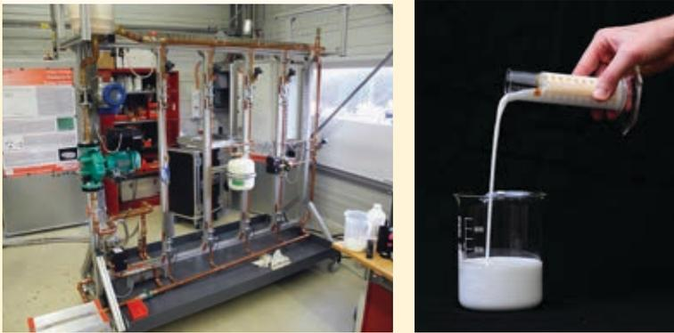
Fig. 4 Test rig for testing the dispersions with different heating technology components
