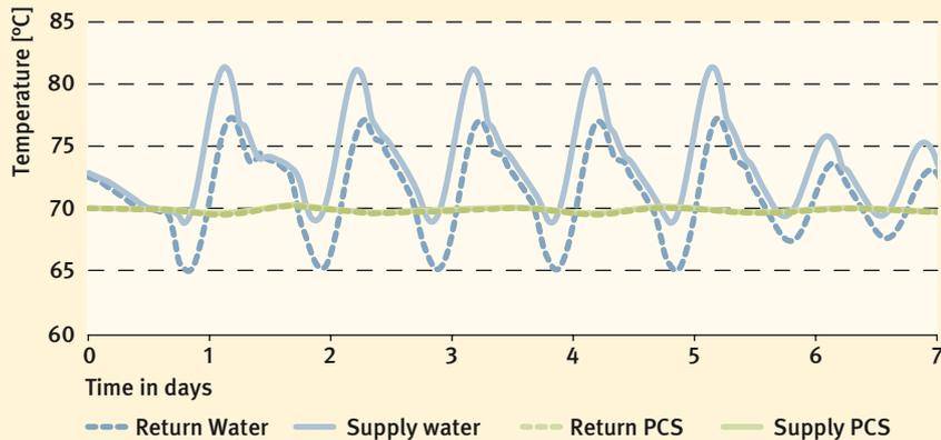
Fig. 2 Supply and return temperatures for the district heating network for water and the paraffin-water dispersion
