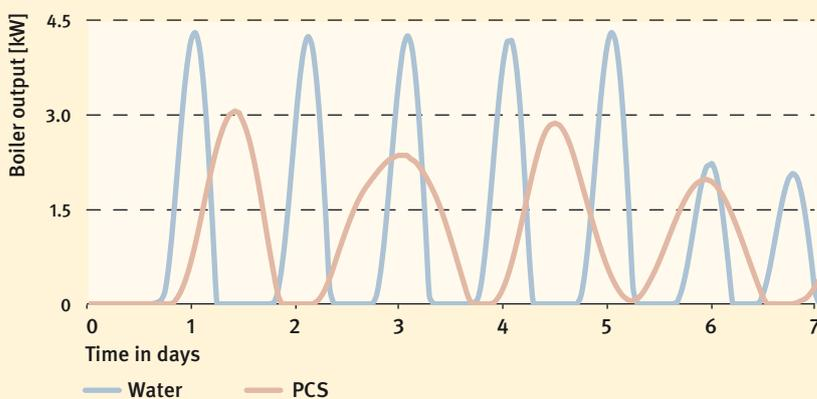
Fig. 5 Comparison of the boiler output for the heating network for water and the paraffin-water dispersion
