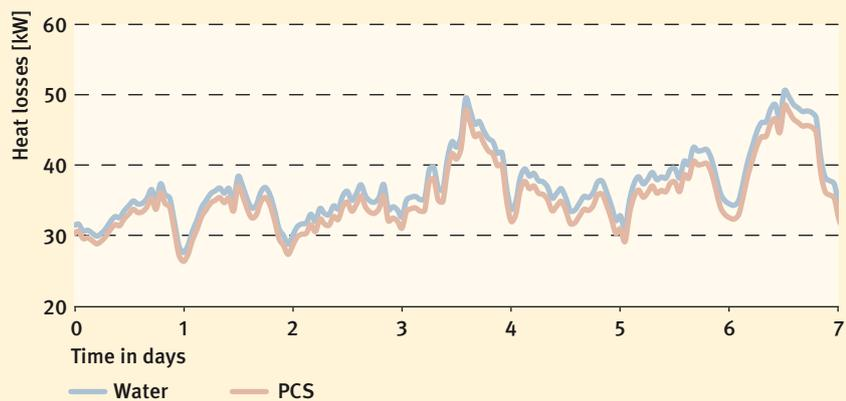
Fig. 3 Heat losses from the district heating network for water and the paraffin-water dispersion
