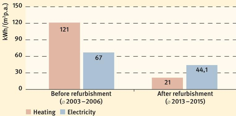
Fig. 3 Average final energy consumption measured for heating and electricity before and after renovation
