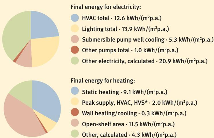
Fig. 4 Distribution of the measured consumption of electricity and heat energy (2014). Some of the electrical loads are not recorded separately, such as the electricity consumed by lifts, individual pumps and users. Heating, ventilation and sanitation (HVS)\* manuscript reading room
