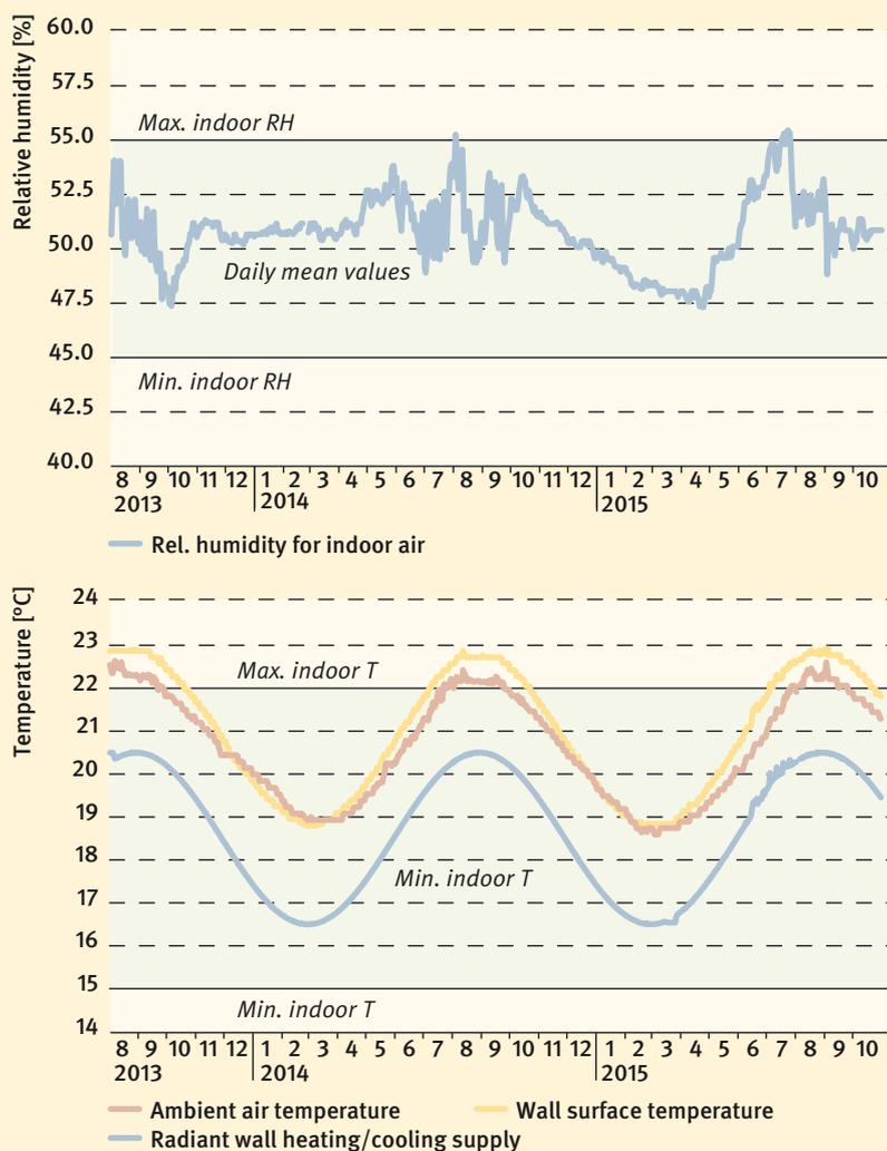
Fig. 2 Measurement results for the indoor environment in the manuscript stacks in the basement, August 2013 to October 2015. The target values for the indoor air temperatures are slightly exceeded by between 0.2 and 0.8 K during the summer months.
