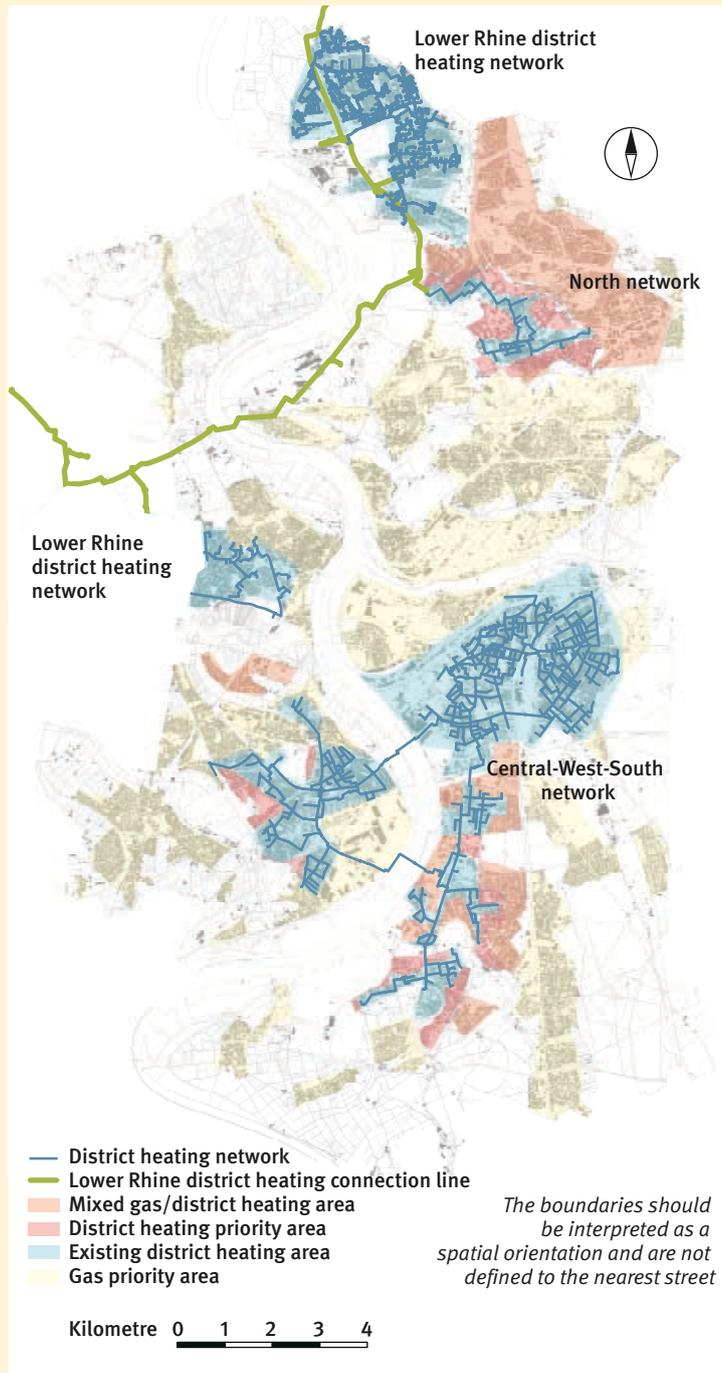
**Fig. 3** In future, the parallel supply with gas and district heating is to be reduced. In an initial design, the experts have demarcated supply areas for this purpose.
