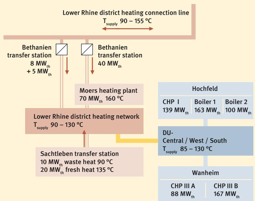
Fig. 2 This is how the connection between the Lower Rhine district heating connection line and the Duisburg Central/West/South network could look like.
