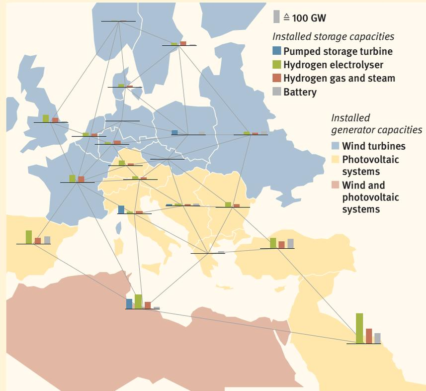
Fig. 1 The graphic shows an overview of the base scenario. Regions coloured blue represent the use of wind energy, yellow the use of photovoltaics. In North Africa both technologies are used.
