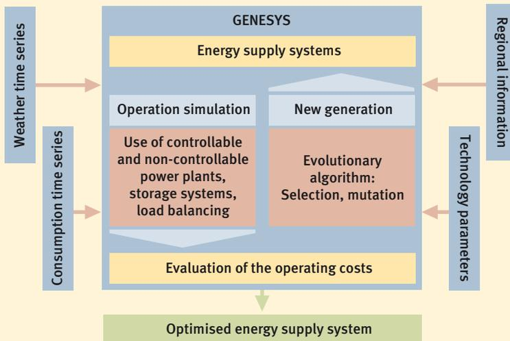
Fig. 4 The flow chart explains the evolutionary system optimisation using the example of the GENESYS program. The input time series are available in hourly resolution.
