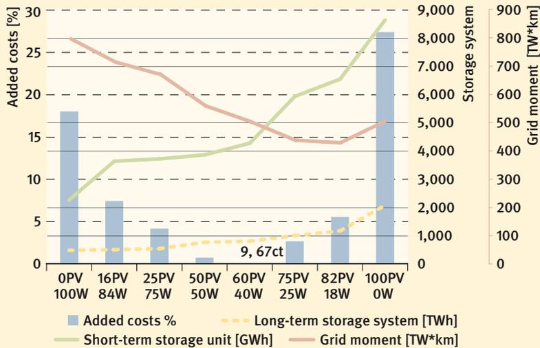
Fig. 3 The respective variations in the relative production capacity show the additional costs relative to the base scenario and the changes in terms of the storage requirements and grid moment.
