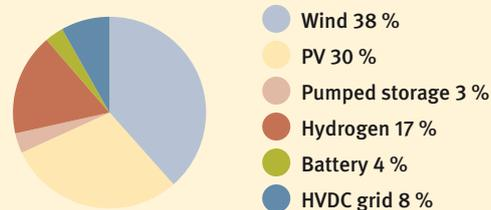
Fig. 2 The pie chart shows the percentage cost distribution in the base scenario. 30 % of the energy generation costs are caused by PV generation and 38 % are caused by wind generation. Storage systems cause 24 % of the costs and networks 8 % of the costs.
