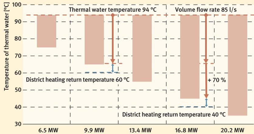
Fig. 1 The graphic shows the geothermal heat output in accordance with the reinjection temperature of the thermal water.
