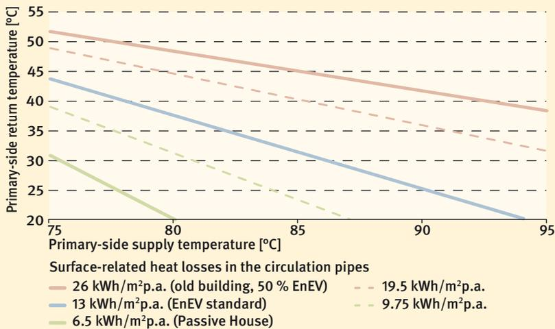
Fig. 3 Possible primary-side return temperatures at a district heating transfer station (DHTS 3) with indirect connection in summer mode (without heating) in accordance with the primary-side supply temperature and the area-related heat losses in the circulation pipes
