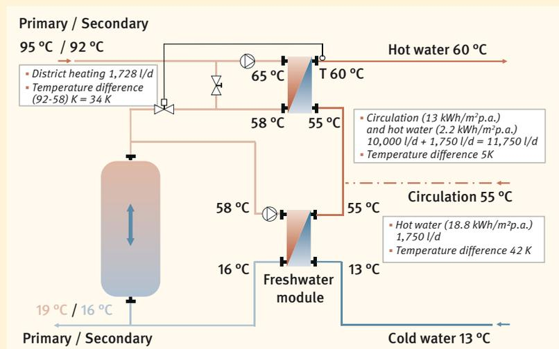
Fig. 2 Principle behind cascaded domestic hot water heating with an ideally stratified heating buffer storage tank (DHTS 3): In pure circulation operation, the buffer storage tank is charged and then discharged with high hot water consumption. The numerical values correspond to an apartment building with 20 residential units.
