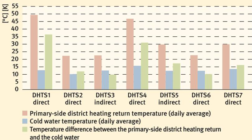
Fig. 4 Daily averages of the primary-side return temperatures for the investigated district heating transfer stations in summer mode (without heating) with well-insulated circulation pipes (to EnEV standard) and a primary-side supply temperature of 95 °C
