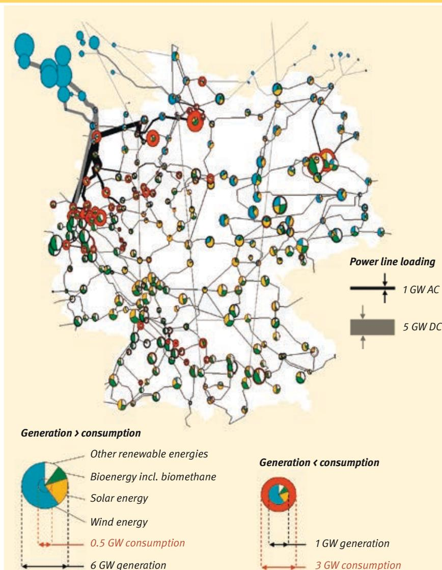
Fig. 1 Illustration of the topological distribution of grid nodes in Germany with the corresponding ratio of offered to demanded energy.
