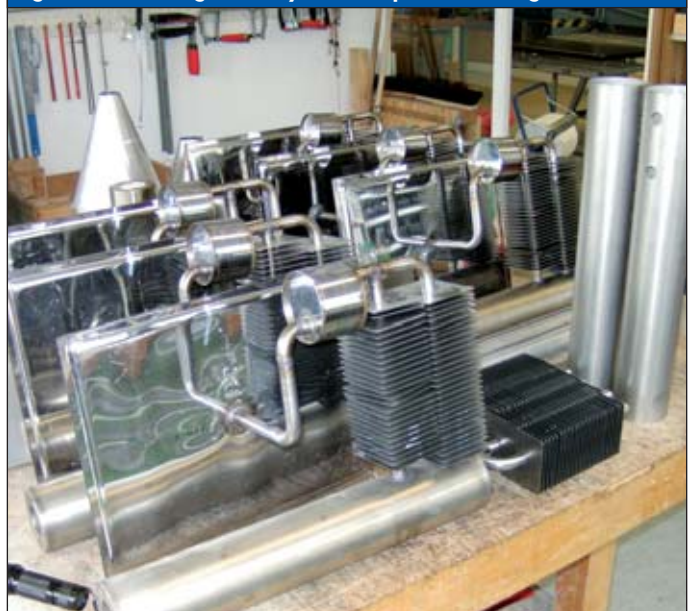
Fig. 5: Zeolite refrigeration systems for practical testing
