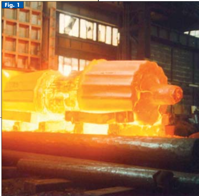
A generator shaft for a power plant leaves the reheating furnace of a hammer forge.
