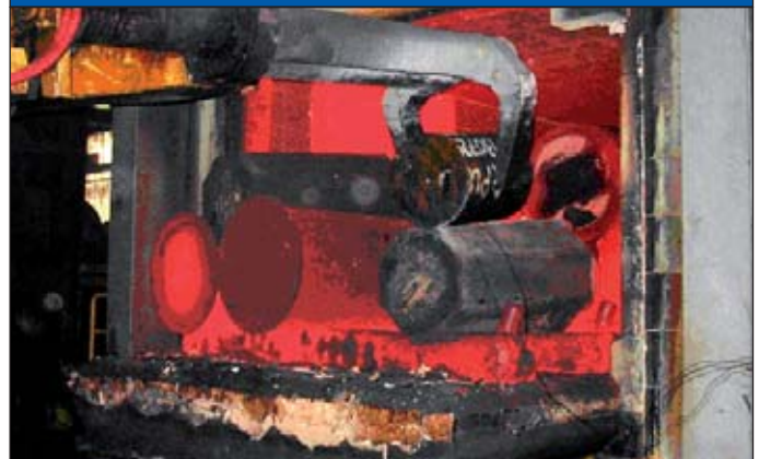
Fig. 8: Through-heating measurement with trial ingot
