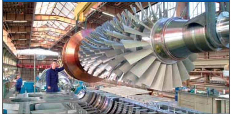
Fig. 5: Axial-radial compressor, suitable for the low pressure component (LP in fig. 4)
