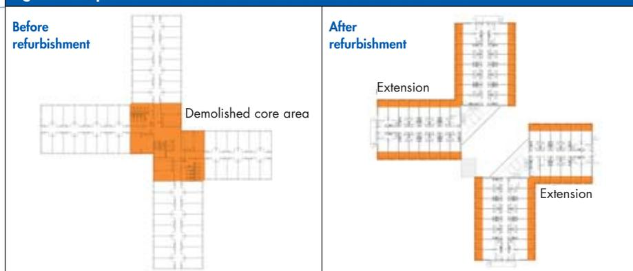
Fig. 4: Initial state and realised refurbishment, planning data
