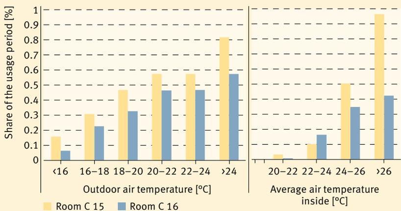
**Fig. 4** Use of the ceiling fans depending upon the outdoor or indoor air temperatures during the usage period. In the event of indoor air temperatures over 26 °C, the ceiling fan was activated for up to 97 % of the usage period.
