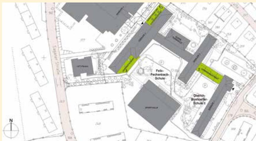
Fig. 1 Site plan: The extensions (an administration area, a learning area and a teaching restaurant) that were built prior to the refurbishment are marked in green.
