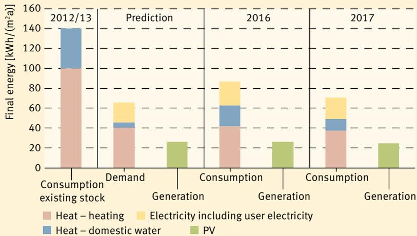
**Fig. 3** Annual balance of the final energy in comparison to existing building stock and the demand predictions (based on the reference climate in Potsdam); there is no energy consumption measurement data for the existing stock. Thanks to the primary energy factor of 0 for the district heating, the solar power, which is mainly used on site, and the refurbishment of the building envelope an energy plus level has been achieved.
