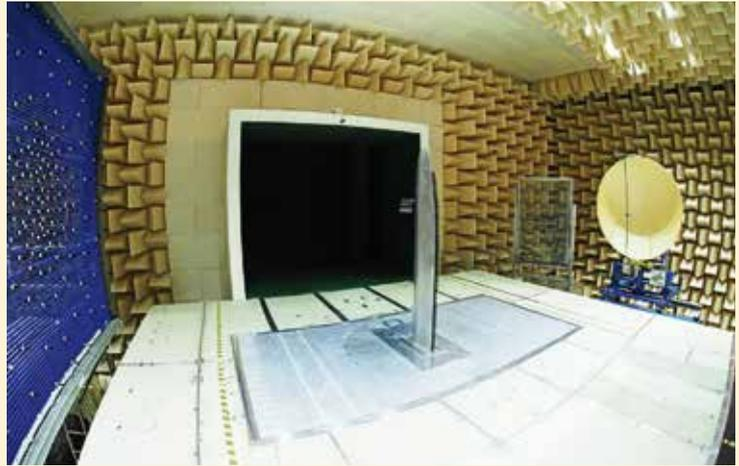
**Fig. 1** The measurement of the noise sources is performed in the wind tunnel (DNW-NWB) using a directional microphone arrangement (elliptic mirror) and 2 measurement arrays: The left field has a diameter of 3 m, 140 microphones and is facing the suction side. The right field has a diameter of 1 m, 96 microphones and is located next to the mirror on the pressure side. Measurement object is an airfoil with brush extension.
