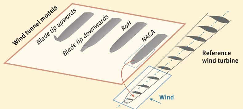
**Fig. 2** Overview of the tested model variants without trailing edge modifications. The two left blade tips on the wind tunnel models show winglets bent up and down.
