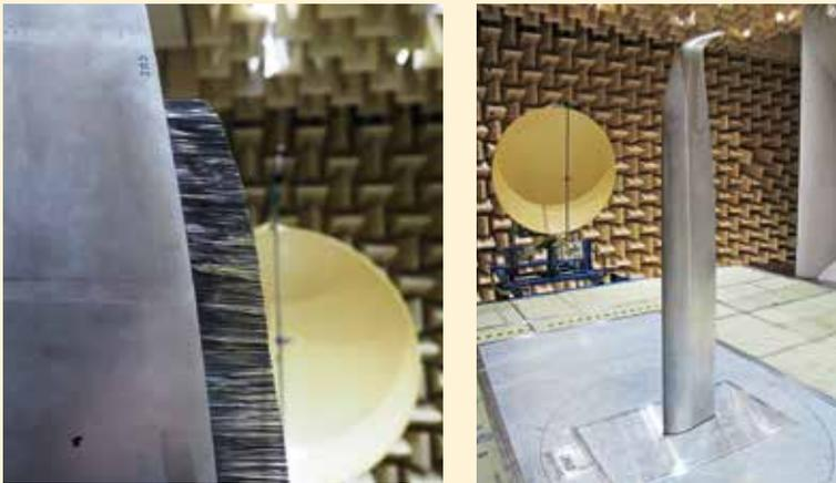
Fig. 3 A modified trailing edge with brush extension – model configuration with winglet
