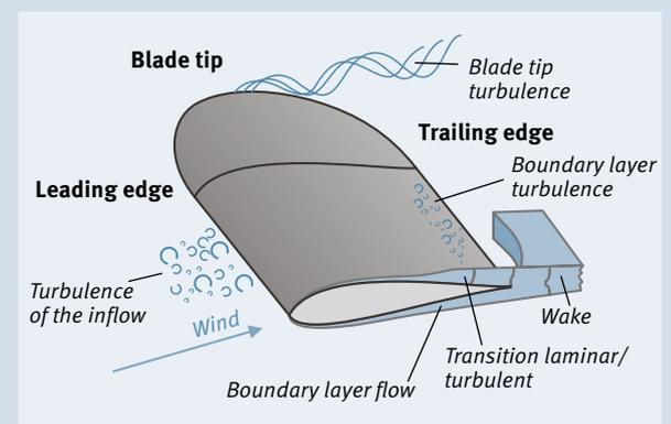
Fig. 5 Noise sources on the rotor blade with boundary layer flow around a profile (boundary layer thickness is vastly elevated)
