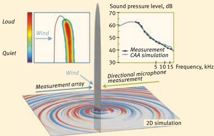
Fig. 4 “Snapshot” of the sound field from 2D simulation of trailing edge noise (bottom). Example of source map from array measurement at 2.5 kHz with line source distribution along on the trailing edge (top left) and comparison of measured vs. simulated noise spectrum (top right).
