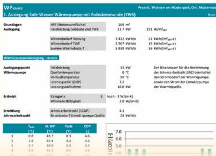
Fig. 4 WP<sub>SOURCE</sub> software (only in German available) can be used to evaluate heat exchangers for specific buildings and commercially available heat pumps.
