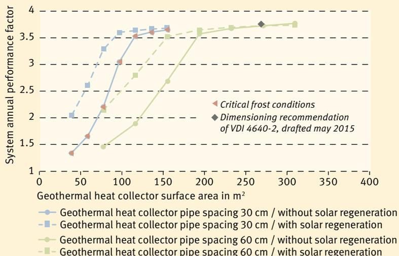
Fig. 1 System annual performance factors ( $APF_{sys}$ ) dependent on size of geothermal heat collector, solar regeneration and layout spacings in geothermal heat collector
