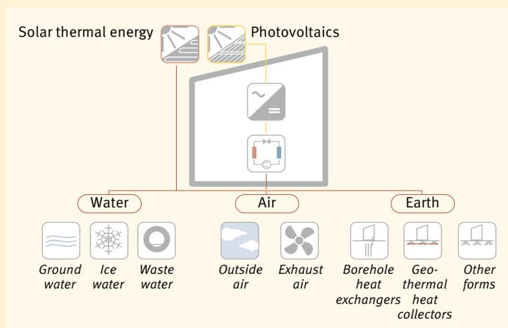
Fig. 2 Many heat sources and heat exchangers exist. Each project involves identifying the optimal configuration.
