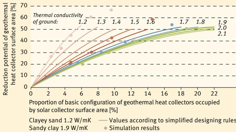
Fig. 3 The surface area of the geothermal heat collector can be reduced in size as the solar collector surface area increases – dependent on the thermal conductivity of the ground (in W/mK).
