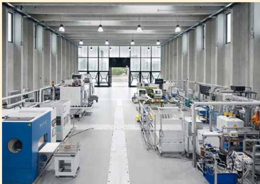
Fig. 1 In the ETA Factory, the production machines and building are networked energy efficiently and unavoidable waste heat continues to be used in the system.
