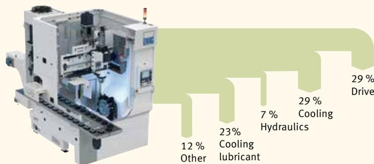
Fig. 2 Where the deployed energy flows: Active power requirement of a lathe.
