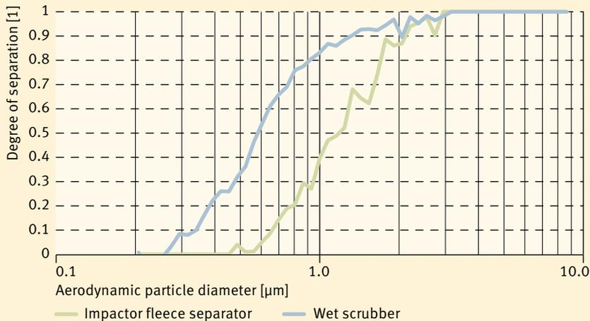
Fig. 3 Comparison of the separation efficiency of a scrubber and a standard impactor-fleece separator, measured on a 4-cylinder diesel engine.
