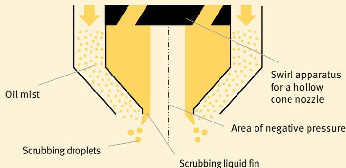
Fig. 1 Schematic depiction of the operation of a wet scrubber
