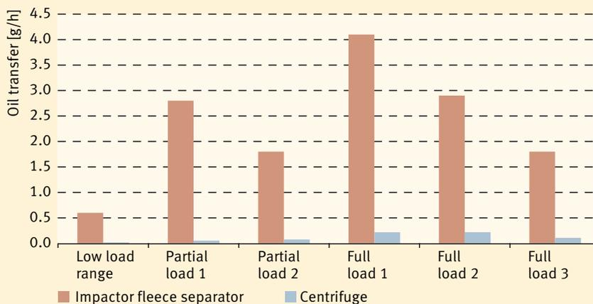
Fig. 4 Comparison: Separation performance of a disc centrifuge and standard impactor-fleece separator, oil discharge measured on a 4-cylinder diesel engine.
