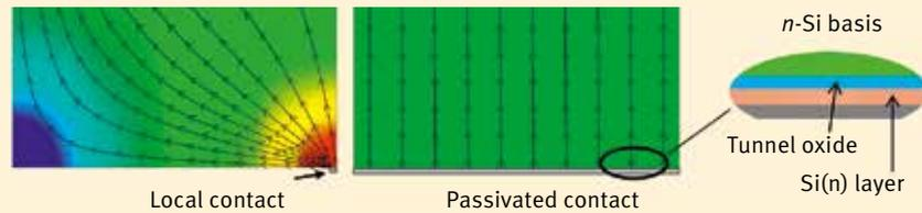
Fig. 1 The simulation shows the difference between the electrical current transport in solar cells with local backside contacting (left) and in cells with the new, full-area passivated TOPCon backside contact (right).
