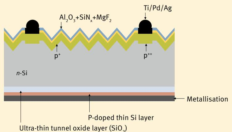
Fig. 2 Schematic diagram of the TOPCon (Tunnel Oxide Passivated Contact) solar cell with full-area selective contacts.
