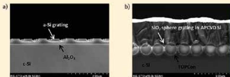
**Fig. 4** SEM micrographs of the cross-sections through EPOS cells: on the left the crossed grating produced by nanoimprint lithography, on the right the structure on TOPCon cells created using  $\text{SiO}_2$  spheres (each without metallisation).
