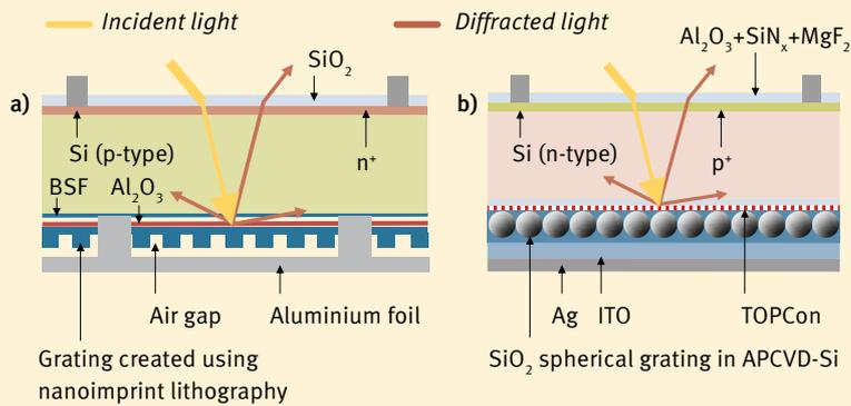
**Fig. 3** EPOS solar cells with diffractive backside gratings: (a) p-type cell with thin  $\text{Al}_2\text{O}_3$  backside passivation and a binary crossed grating in a-Si. (b) n-type cell with a passivated backside contact (TOPCon) and a sphere grating on the rear. Full-area backside contact (ITO/silver).
