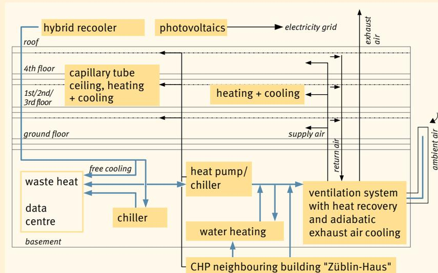
Fig. 1 Technology concept for heating, ventilation and cooling
