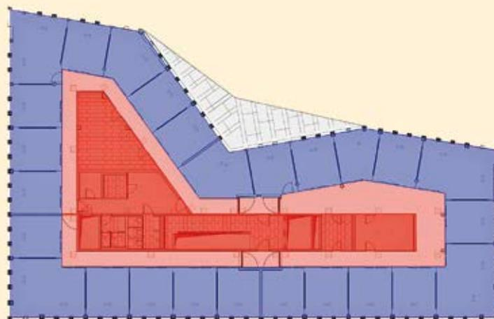
Fig. 2 Floor plan of the third storey: The staircase, corridors, meeting rooms, copy rooms, IT rooms, kitchenettes and toilets are located in the inner zone (red).
