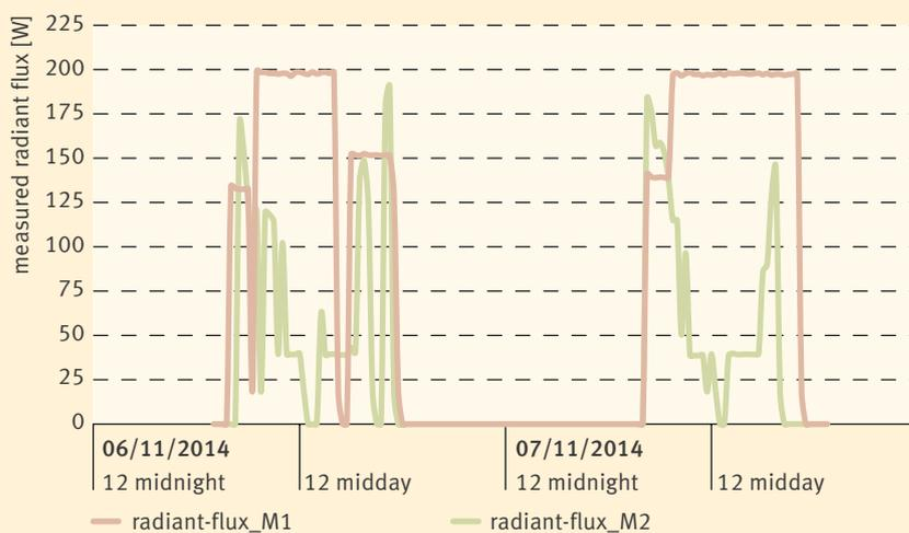
Fig. 4 Comparison of lighting intensity profiles in two test rooms: In room M1, the staff taped off the sensors and parts of the lighting to manipulate the dimming function because they were dissatisfied with its performance.
