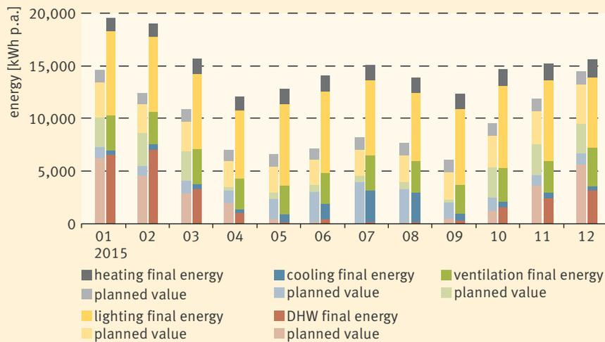
Fig. 3 Final energy consumption 2015 sorted by consumption categories and compared to planned values
