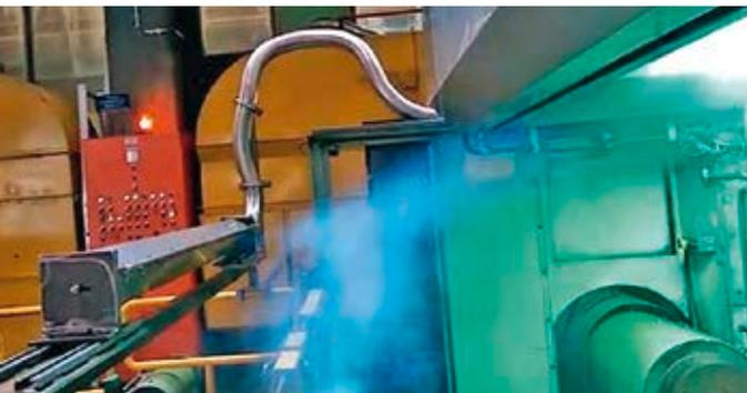
Fig. 1 Injected smoke shows the barrier effect of the air blade.
