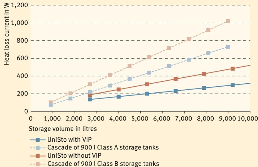
Fig. 1 Compared with storage cascades, the heat loss currents do not increase as much proportionally to the volume in the new storage system. Unlike storage cascades, UniSto storage tanks have lower heat losses the greater the overall volume is. (VIP = Vacuum Insulation Panel)
