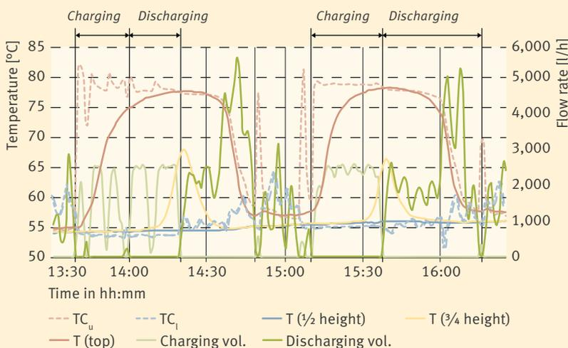
**Fig. 4** Volume flows and storage tank temperatures during operation on 02/01/2016 in the middle storage module of the first demonstration system in Rheinfelden
