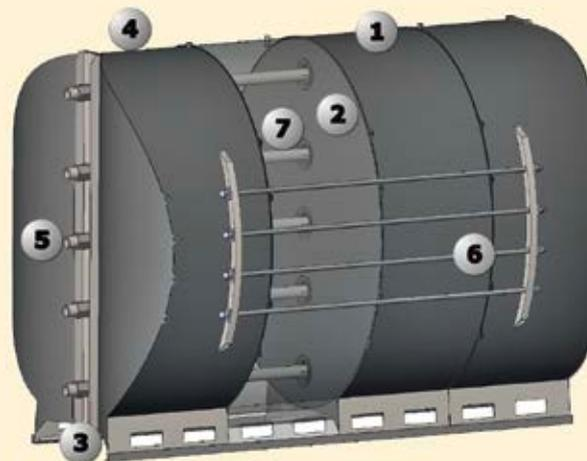
Fig. 2 This UniSto storage tank consists of four modules. The elements in detail: (1) vessel shell, (2) thin steel plate, (3) rails, (4) pressure resistant end modules, (5) charging and discharging pipes, (6) connecting rods, (7) seal system
