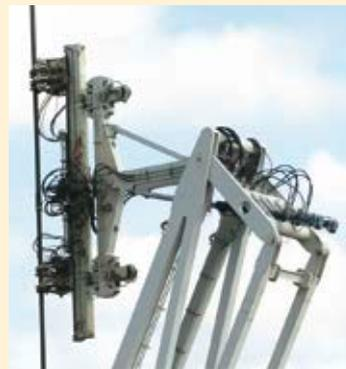
Fig. 5 A pipe handler automatically transports the individual parts of the drill pipe from the store to the drill drive. This reduces noise emissions.
