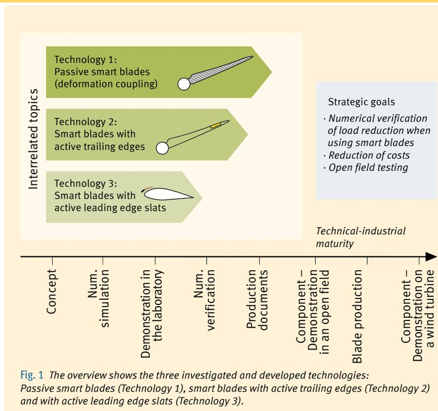
Fig. 1 The overview shows the three investigated and developed technologies: Passive smart blades (Technology 1), smart blades with active trailing edges (Technology 2) and with active leading edge slats (Technology 3).
