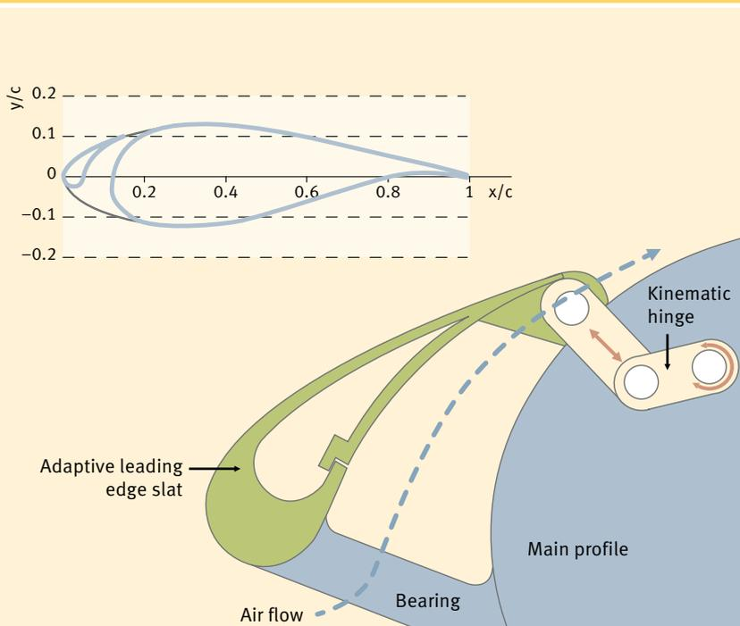
**Fig. 4** Optimal geometry: The integrated leading edge slat (top) was experimentally tested in wind tunnel tests. As a second variant, the original profile of the reference blade was retained and the leading edge slat was placed on the profile (bottom)
