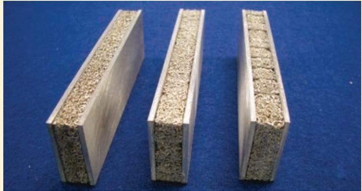
Fig. 2 In addition to metal foams, selected fibrous structures were also produced as sandwich samples for the heat transfer measurements
