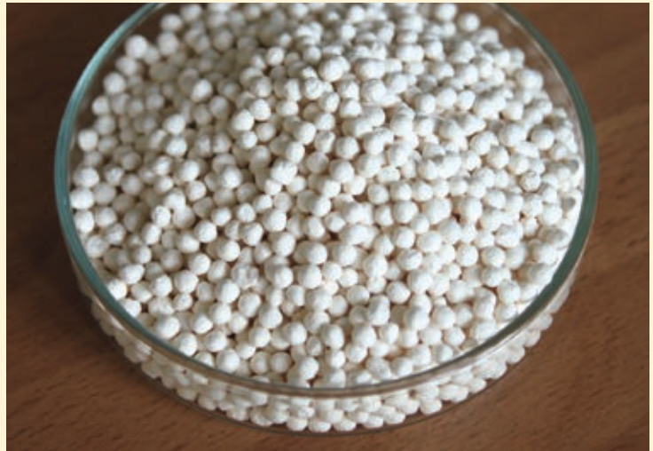
Fig. 2 Zeolite beads without a binder have a greater active mass and surface area
