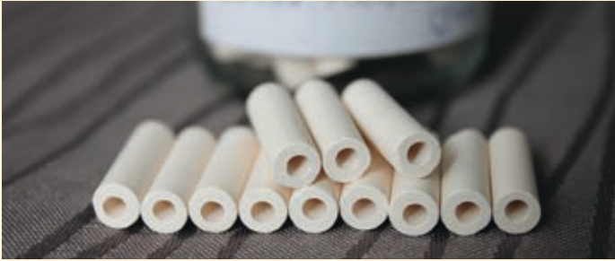
Fig. 4 Zeolite extrudates made of pure zeolite A in the form of macaroni
