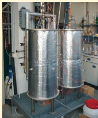
Fig. 7 The two zeolite containers are alternately charged and discharged.
