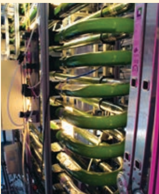
Fig. 6 An algae reactor utilises CO 2 and heat from the CHP exhaust gas.
