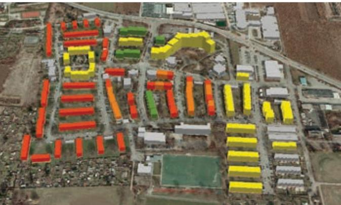
**Fig. 1** Heat requirement simulation for the existing Grünbühl district using a 3D urban model.
