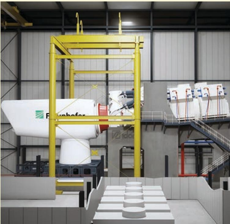
Fig. 4 The test rig drive is mounted on a concrete foundation. The nacelle is fixed to this foundation via a pallet system.
