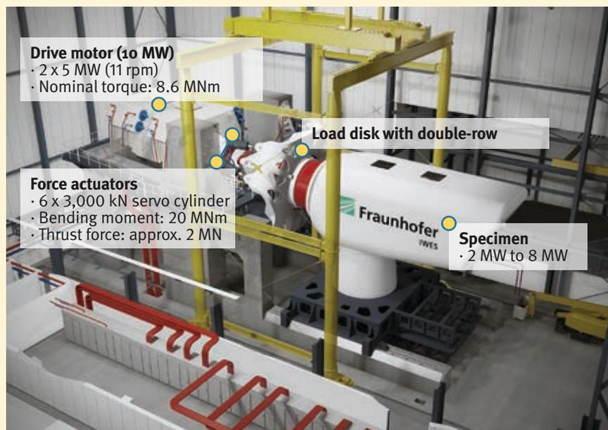
Fig. 1 Load transmission: six hydraulic cylinders transfer the forces and moments to the nacelle. The electricity grid is modelled in the converter room behind.
