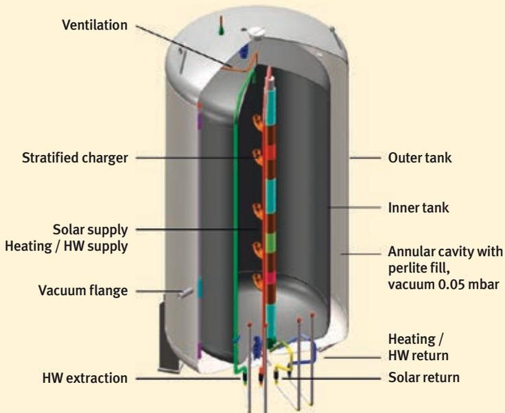
Fig. 3 Schematic view of a VSI storage tank
