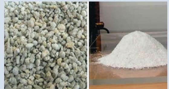
Fig. 5 Rough grained crude perlite (left) and technically expanded perlite.
