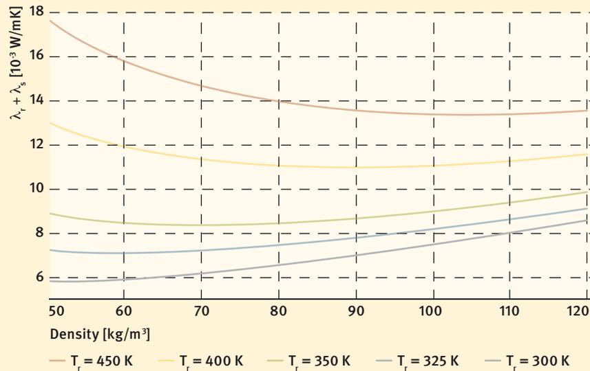
Fig. 1 The thermal conductivity of the evacuated tank shell consists of radiation ( $\lambda_r$ ) and solid-state thermal conductivity ( $\lambda_s$ ) and is dependent on the density and average temperature ( $T_r$ ) in the perlite filling.
