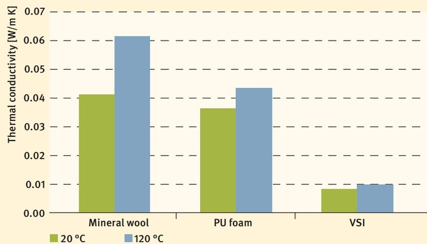
Fig. 2 Comparison of thermal conductivity of conventional insulating systems with innovative VSI insulation at  $20\text{ }^{\circ}\text{C}$  and  $120\text{ }^{\circ}\text{C}$  average temperature.
