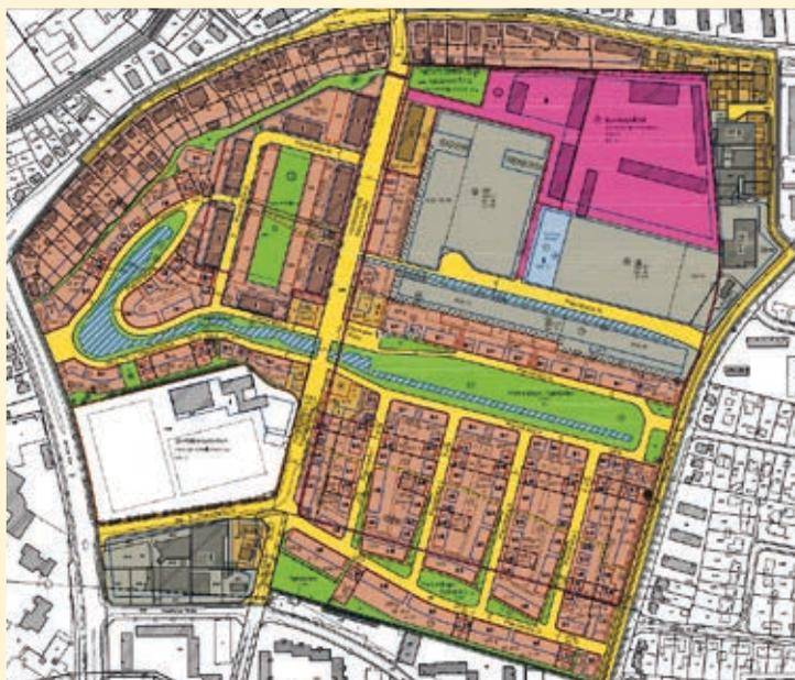
Fig. 2 The Jenfeld 23 land-use plan designates the residential, mixed, core and commercial areas (brown, red and grey colours) as well as the HAMBURG WASSER operational facility (blue colour) in the commercial area.
