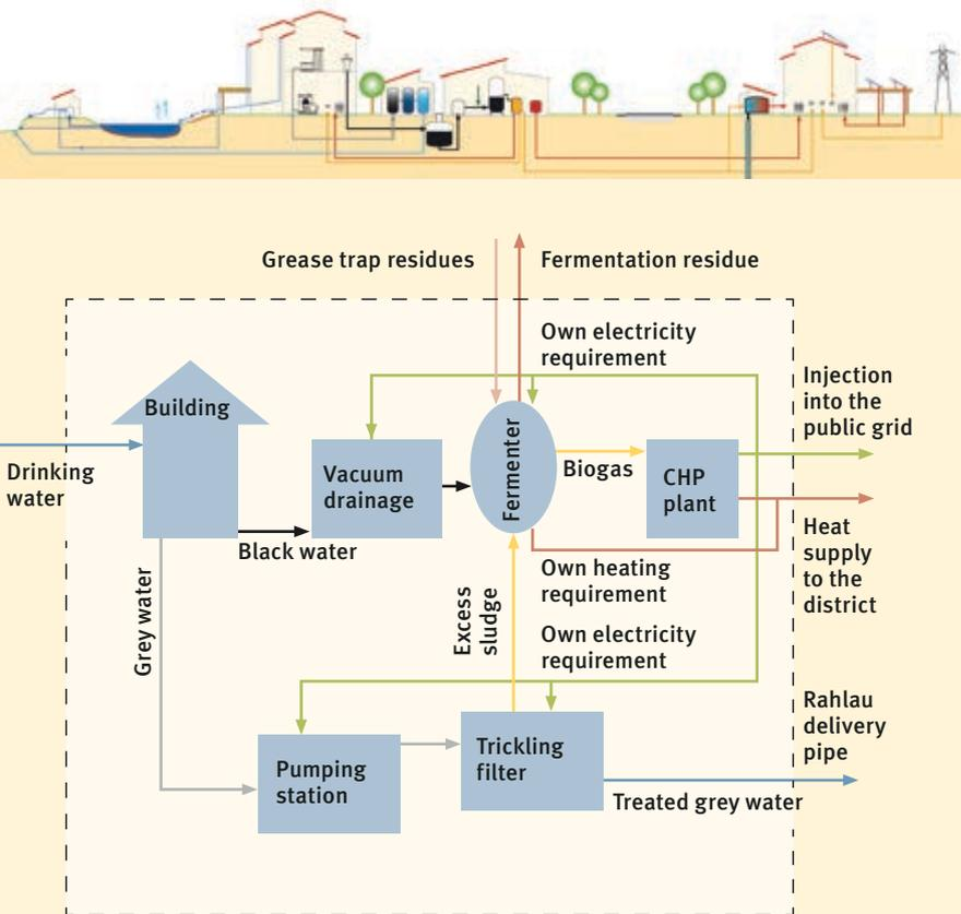
Fig. 3 The illustration and schematic diagram explain the energy recovery and waste water utilisation concept.
