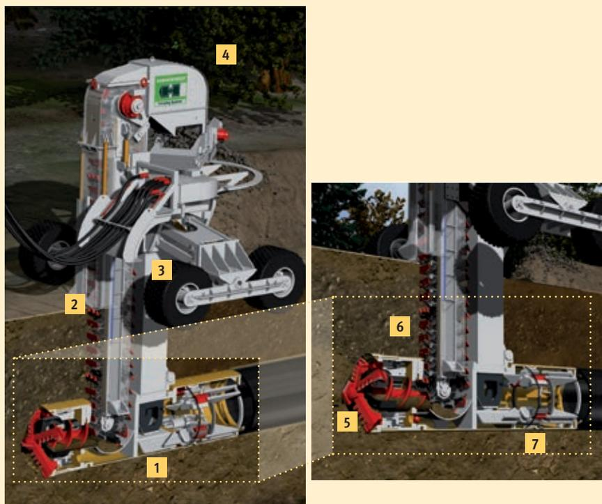
Fig. 2 The excavator unit consists of a tunnel boring machine (TBM) (1), milling unit (2) with buggy (3) and conveyor belt (4). The cutterhead (5) loosens the ground and transports it via the screw conveyor (6) to the milling unit. The steering cylinders (7) are connected with the machine pipe.
