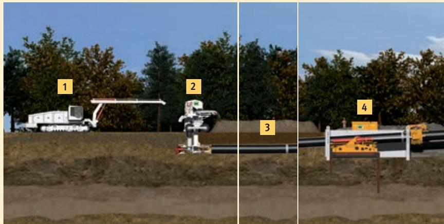
Fig. 1 The operator vehicle (1) controls and monitors the system. The excavator unit (2) loosens the ground and conveys it directly to the surface. The pipe thruster (4) simultaneously pushes the pipeline (3) into the borehole.
