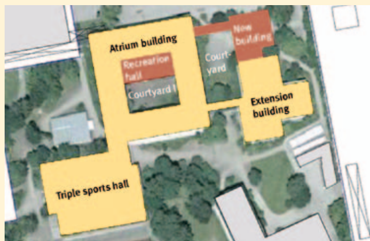
Fig. 1 The construction measures at Marktobendorf Secondary School: The two new parts are marked in red, while the existing buildings undergoing refurbishment are marked in yellow. The existing atrium building is being supplemented with a recreation hall on the courtyard side. The new extension creates a second courtyard as a playground. The newly gained space enables the school to improve the infrastructure for all-day schooling and to restructure the specialist rooms in a sensible manner. Source: Löhle Architekten
