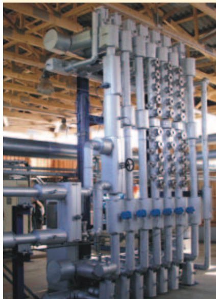
Fig. 1 Test track for corrosion investigations and monitoring.
