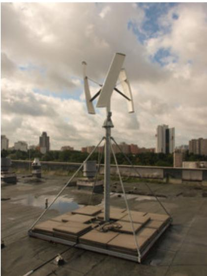
A typical small wind turbine mounted on a roof
