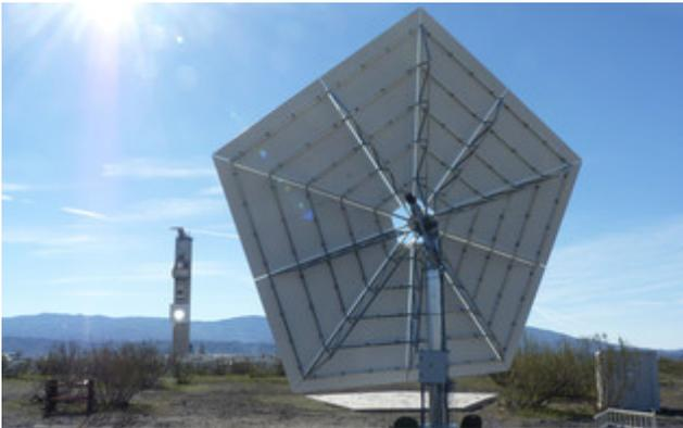
The Stellio heliostat reflects the solar radiation to the solar tower 400 metres away.
