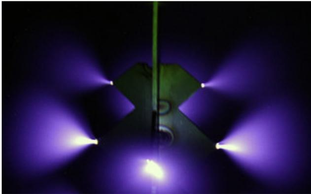
Corona deployed on the discharge electrode
