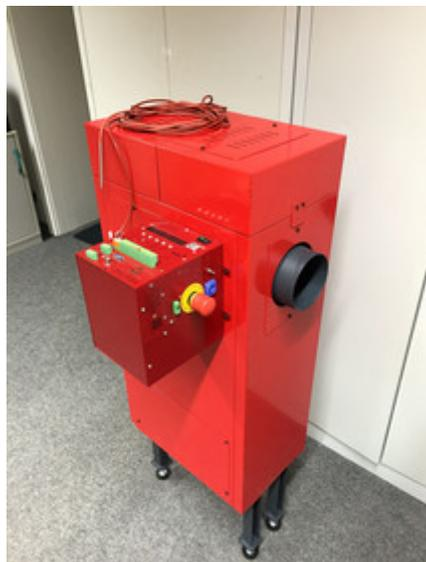
EFC203 electrostatic precipitator system with small precipitator box
