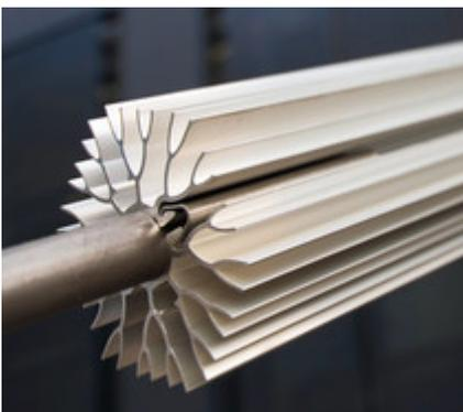
Heat exchanger pipe. The heat is transferred to the salt via the fin structure.
