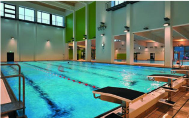
The thermally optimised building envelope makes it possible to operate the passive house swimming pool with higher indoor air humidity without the water condensing on the building components. This means that less water evaporates and both the heating requirement and the need to dehumidify the air in the swimming pool hall are considerably reduced.
