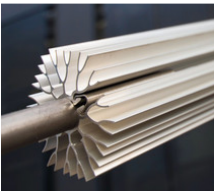
Heat exchanger pipe. The heat is transferred to the salt via the fin structure. © DLR
