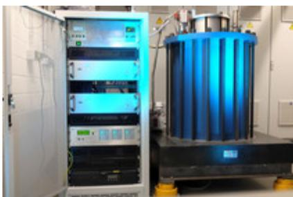
The kinetic energy storage device with innovative external rotor design serves to smoothen the electrical load profile and makes it possible to reduce the connected load of the
