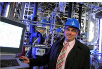
Engineer Alexander Schraven uses more than 50 measurement sensors to record data for characterising the scrubbing liquid.
