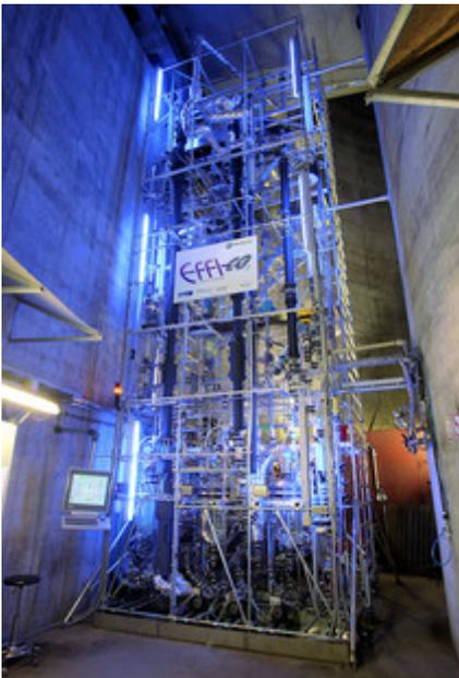
The engineers are testing new scrubbing liquids for capturing CO<sub>2</sub> on the nine-metre-high test rig at the base of the chimney shaft.
