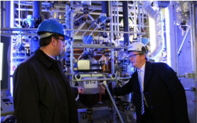
The engineers Alexander Schraven (left) and Matthias Schneider are coordinating the tests with the scrubbing liquids for capturing CO<sub>2</sub> in the test rig at the Herne CHP plant.
