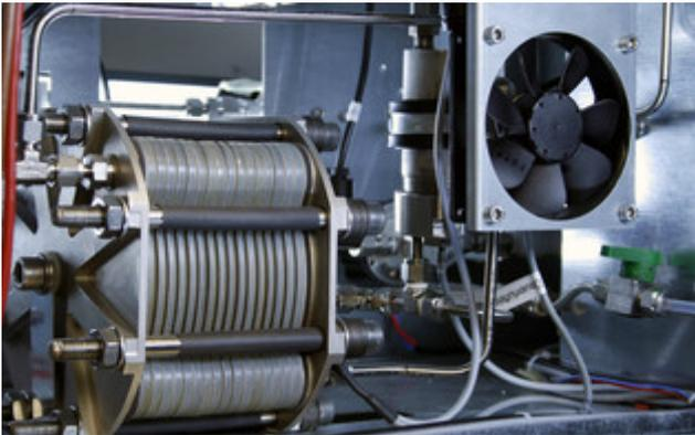
Membrane electrolysis cell stack in a prototype of a pressure electrolyser developed at Fraunhofer ISE
